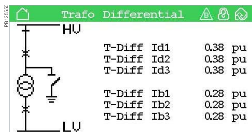
Single line diagram for Transformer Differential application.
